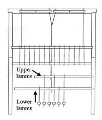
If the weight is not the same, the heavy side falls and it is hard to lift that side.
