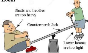
On the Glimakra looms in these diagrams, one pair of shaft bars, 100 heddles and one upper lamm have a combined weight of approx 1 lb.
